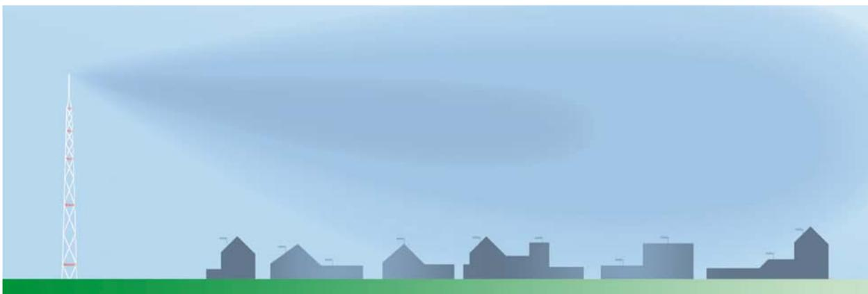
Antennas of large transmitters are installed on high masts in order to improve the range and the antenna beams are designed to achieve as evenly distributed transmission to various distances as possible. This is why the power density at the ground level is low even near the mast.
